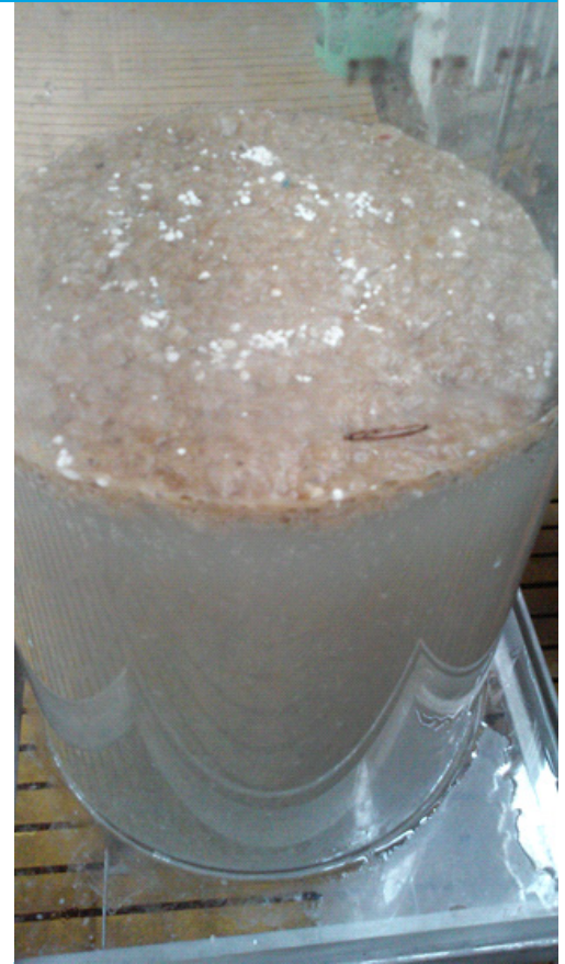
Hydrophobic contaminants from a brown stock mill water sample floating near the surface of the Bubble Nucleation Process Tube. Photograph courtesy of Doshi & Associates, Inc. and the USDA Forest Products Laboratory
